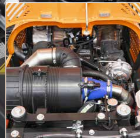
MOTORE YANMAR DA 60 CV STAGE V YANMAR ENGINE 60 HP STAGE V
